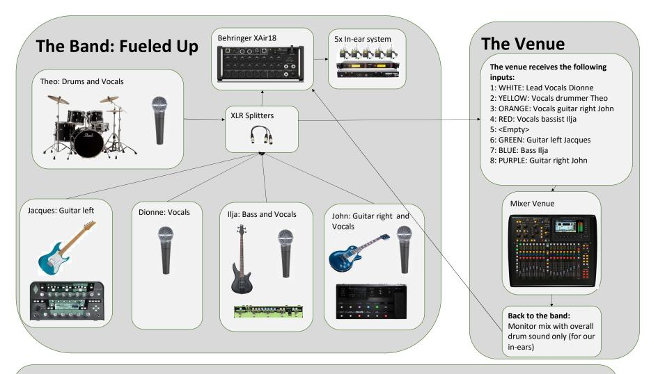
The band has no amplifiers on stage and does not need monitors. All signals from the vocals, bass and guitars go through splitters to both our Behringer XAir18 and the FOH mixer. Up to our Behringer XAir18, we use our own XLR cables. If our Behringer XAir18 can be put close to the sound engineer's stage block or rack, then the splitters are long enough to connect. If that is not possible, we assume that the sound engineer has his own XLR cables to extend connections.
